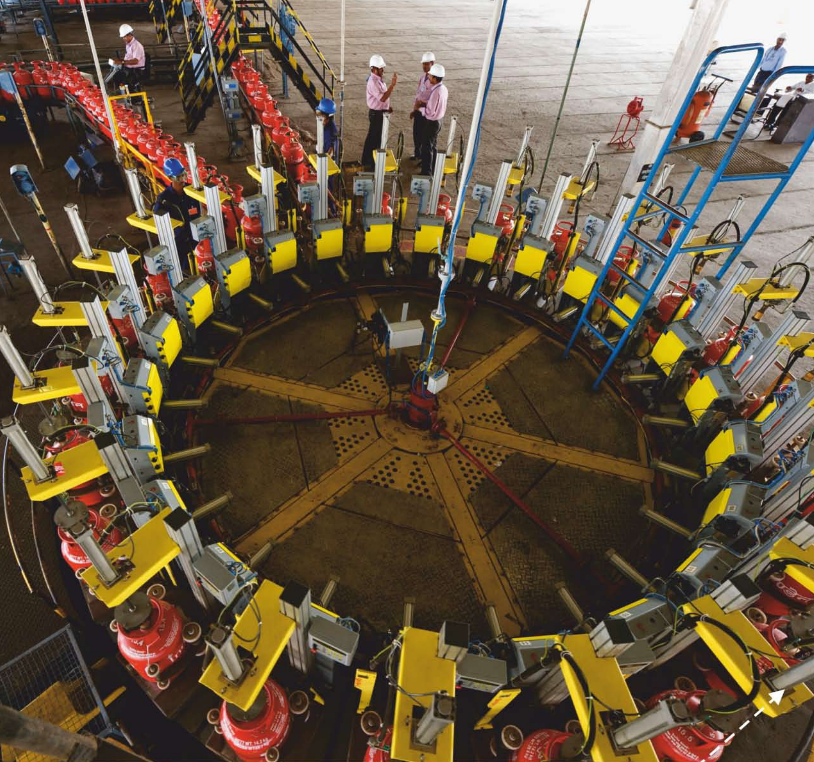
IndianOil's LPG domestic cylinder filling plant
